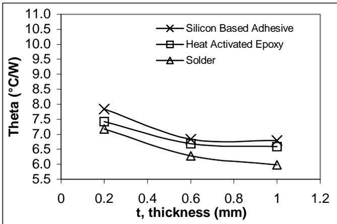
Figure 11. Experimental Thermal Resistance vs. Fin Thickness at velocity of 3.0m/s for Cu 110 Fin
