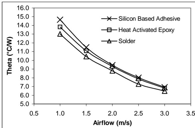
Figure 17. Overall Thermal Resistance (Experimental) of Bonded 0.6 mm Thick Al 3003 Fin
