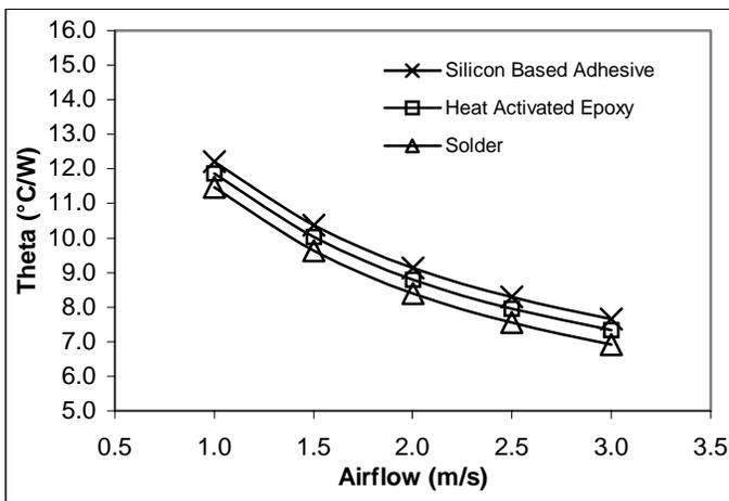
Figure 7. Overall Thermal Resistance (Theoretical) of Bonded 0.2 mm Thick Al 3003 Fin
