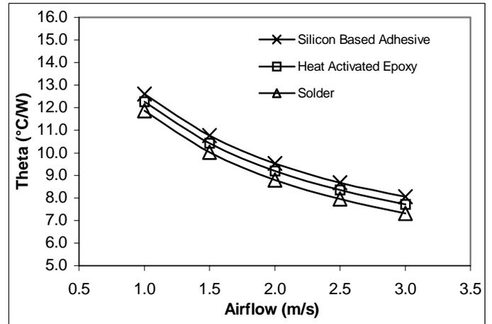
Figure 9. Overall Thermal Resistance (Theoretical) of Bonded 1.0 mm Thick Al 3003 Fin
