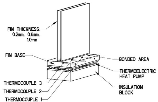
Figure 1. Experimental Setup of Single U-Shape Folded Fin
