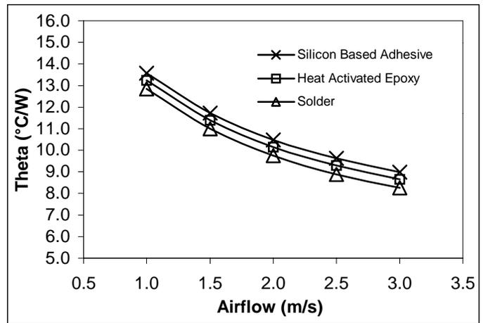
Figure 4. Overall Thermal Resistance (Theoretical) of Bonded 0.2 mm Thick Cu 110 Fin
