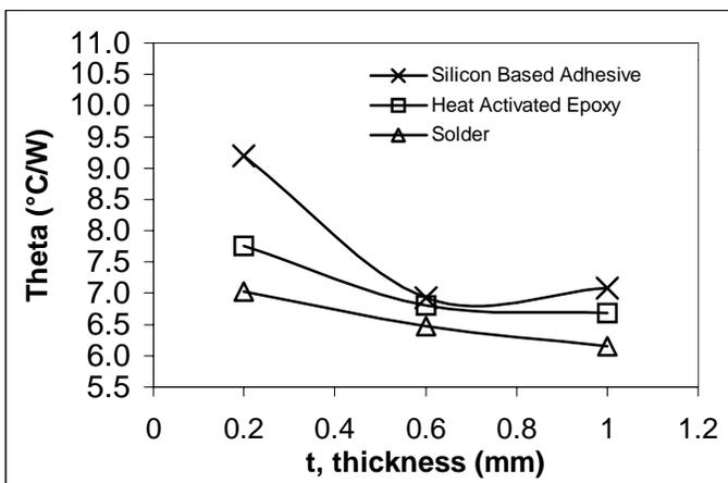
Figure 12. Experimental Thermal Resistance vs. Fin Thickness at velocity of 3.0m/s for Al 3003 Fin
