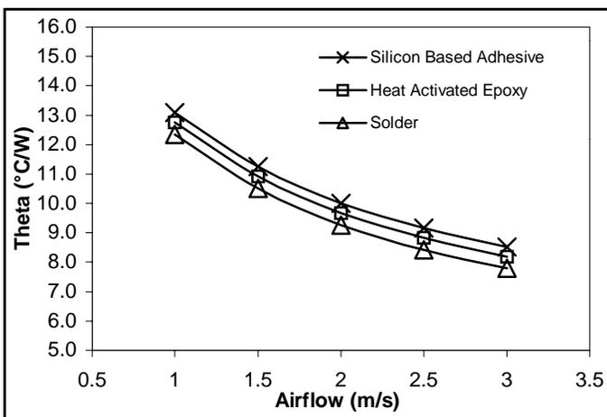
Figure 8. Overall Thermal Resistance (Theoretical) of Bonded 0.6 mm Thick Al 3003 Fin
