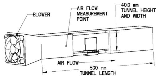
Figure 10. Representation of Bench Top Wind Tunnel
