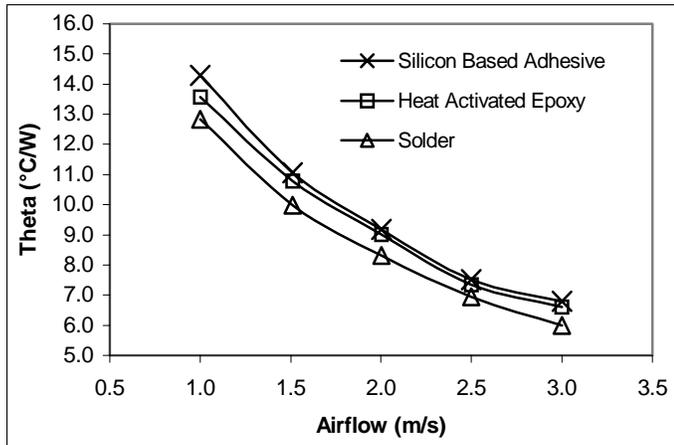
Figure 15. Overall Thermal Resistance (Experimental) of Bonded 1.0 mm Thick Cu 110 Fin
