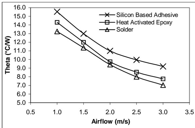
Figure 16. Overall Thermal Resistance (Experimental) of Bonded 0.2 mm Thick Al 3003 Fin
