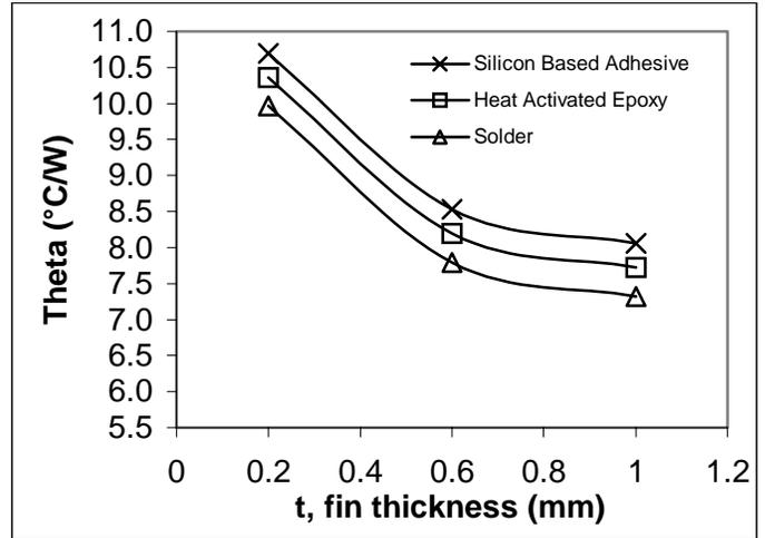
Figure 3. Theoretical Thermal Resistance vs. Fin Thickness at velocity of 3.0m/s for Al 3003 Fin
