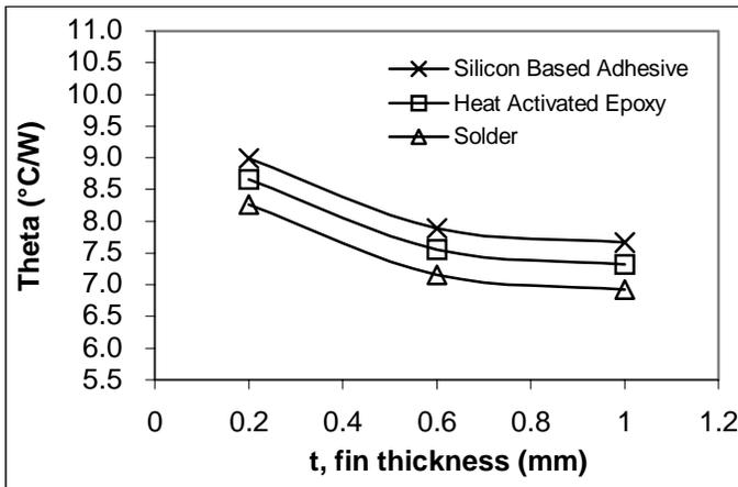
Figure 2. Theoretical Thermal Resistance vs. Fin Thickness at velocity of 3.0m/s for Cu 110 Fin
