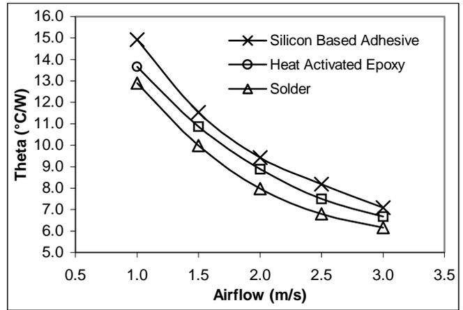
Figure 18. Overall Thermal Resistance (Experimental) of Bonded 1.0 mm Thick Al 3003 Fin
