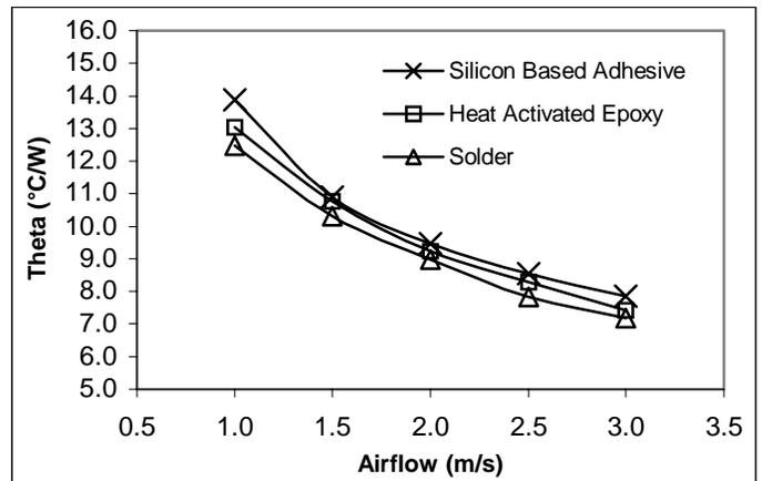
Figure 13. Overall Thermal Resistance (Experimental) of Bonded 0.2 mm Thick Cu 110 Fin
