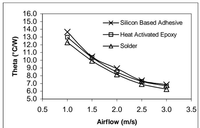
Figure 14. Overall Thermal Resistance (Experimental) of Bonded 0.6mm Thick Cu 110 Fin
