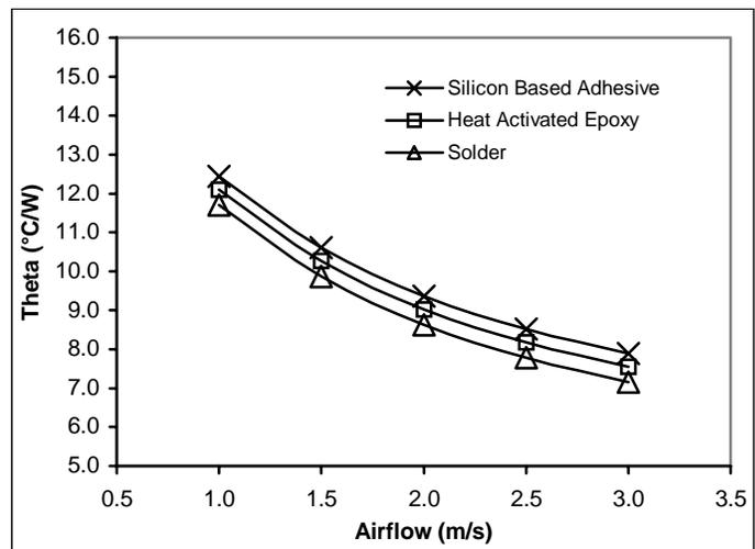
Figure 5. Overall Thermal Resistance (Theoretical) of Bonded 0.6 mm Thick Cu 110 Fin
