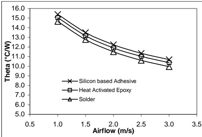
Figure 6. Overall Thermal Resistance (Theoretical) of Bonded 1.0 mm Thick Cu 110 Fin
